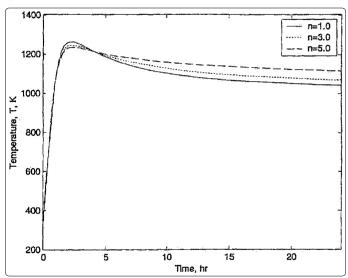
Figure 1. Temperature inside rotary kiln with different number of chlorine atoms and using 10% excess of air where n is the number of chlorine atoms
