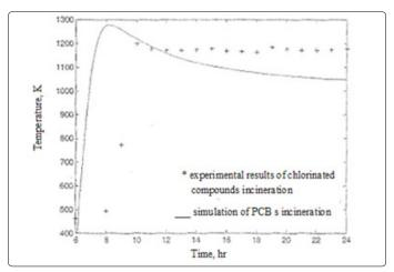
Figure 2. Temperature inside rotary kiln from the current model and compared with experiments
