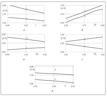
**Figure 4.** Dependences of the sizes Q and  $H_0$  from ε (a) at H=3, L=2,  $H_1=1$ ,  $H_2=1.4$ , from H (6) at ε=0.5, L=2,  $H_1=1$ ,  $H_2=1.4$ ; or L (B) at ε=0.5, H=3,  $H_1=1$ ,  $H_2=1.4$ ; from  $H_1$  (r) at ε=0.5, H=3, L=2,  $H_2=1.4$ ; from  $H_2$  (Д) При ε=0.5, H=3, L=2,  $H_1=1$ .
